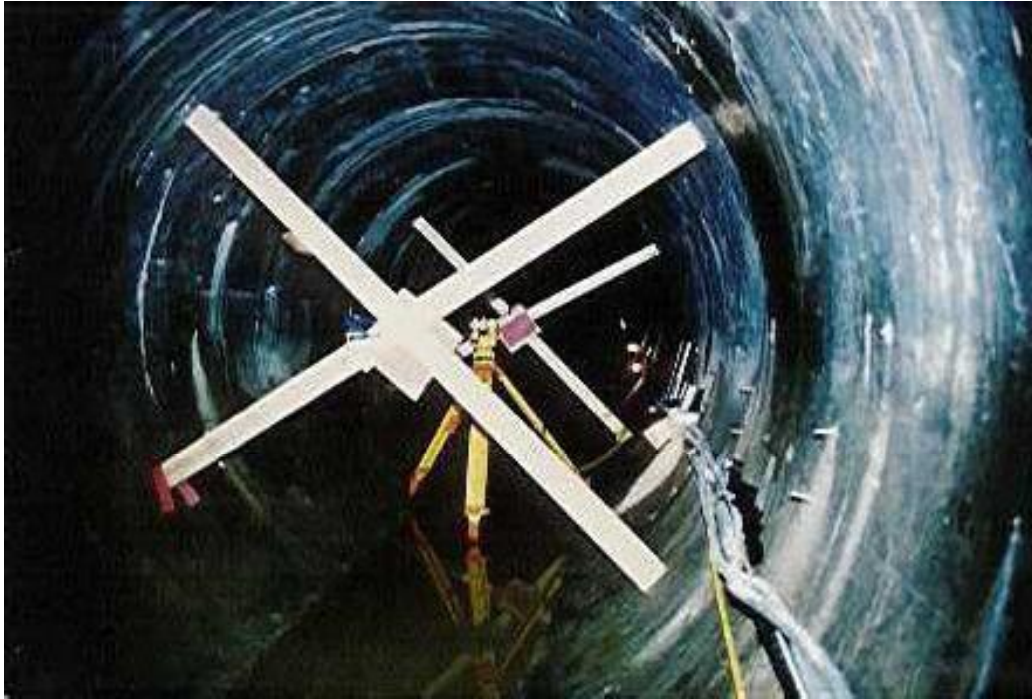
Picture 1: Typical set up for the mechanical theodolite method (courtesy of Accusonic Technologies, Jim Walsh)
