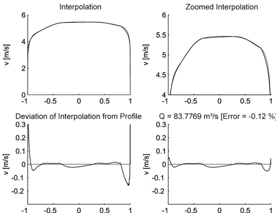
Fig. 8 Comparison of calculated versus measured flow profile
