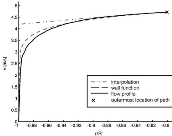
$$v(x, y) = v_{\max} \left( 1 - \frac{\sqrt{x^2 + y^2}}{R} \right)^{1/n}$$
