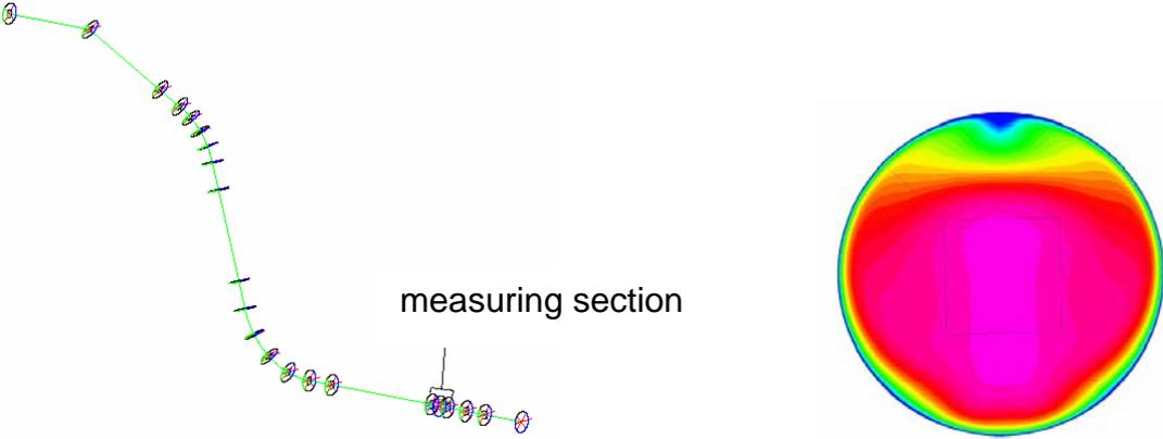
Figure 5 Penstock configuration and flow field
