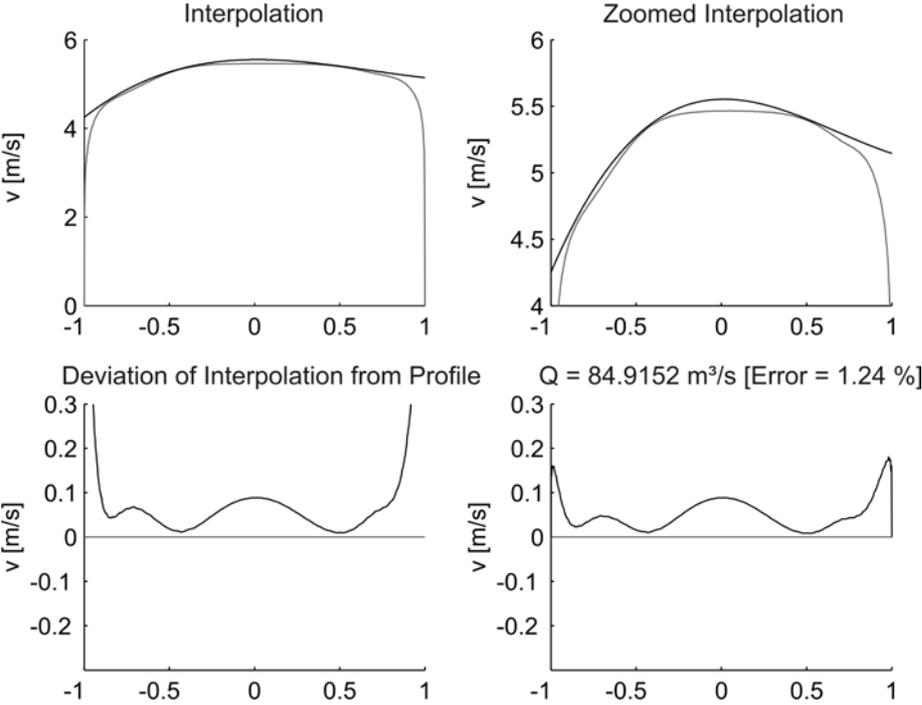
Figure 6 Comparison of calculated versus measured profile (classical method)
