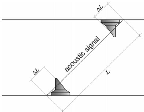
$$\bar{v}_c = \frac{1 - \frac{2\Delta L}{L}}{1 - \left( \frac{2\Delta L}{L} \right)^{1+1/n}} \bar{v}_m$$
