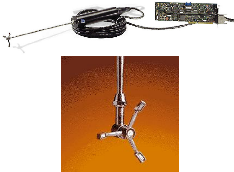
Figure 4: Laboratory version of the ADV. As used at Kennebec, it was equipped with a right-angled head (inset), and the processor board was enclosed in a pressure case, connected to the surface by a power and communication cable.
