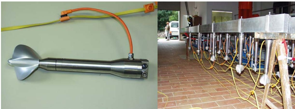
Image (1): Can-Bus-Current Meter and Can-Bus-Current Meter mounted on an aluminium rod ready for installation.
