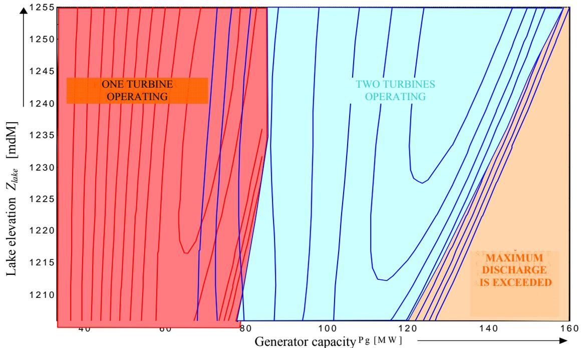
Figure 6 – Station global exploiting characteristic  $\eta_{\text{global}} = \eta_{\text{global}}(P_g, Z_{\text{lake}})$
