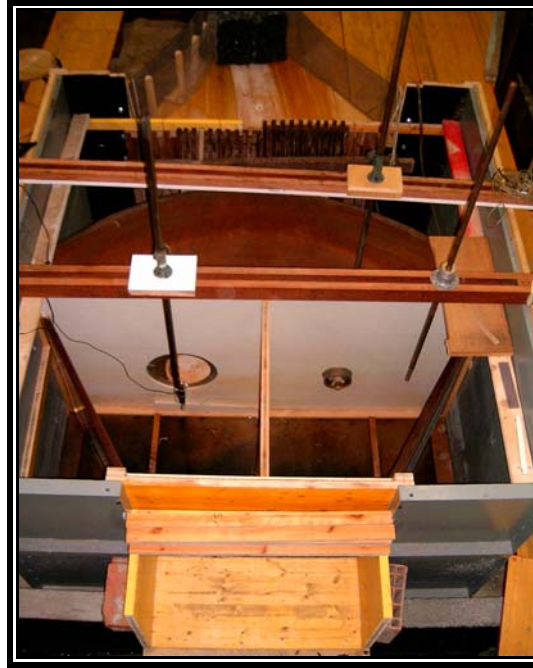
Figure 3 – Calibration tank – from upstream to downstream
