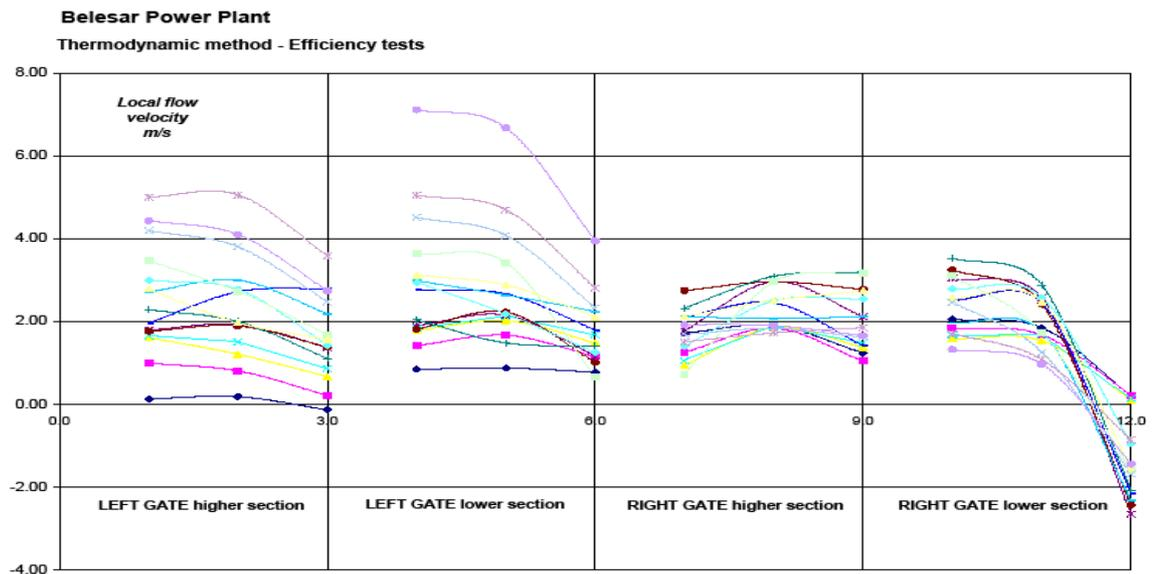
It is noted that the lower right area is affected by phenomena of recirculation marked with negative speed up to 2 m/s recirculation is present since the lower loads, is less affordable for maximum efficiency and return to show very clearly at high flow rates .
