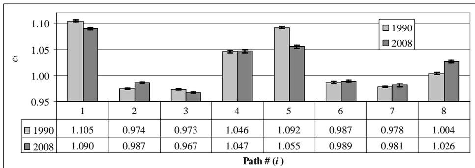
**Figure 3: Coefficients  $c_i$  with random errors measured in 1990 and 2008.**
