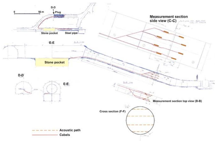
**Figure 1: Detail from drawing of penstock with stone pocket and measurement section. The valve before the spiral casing can be seen on the right.**
