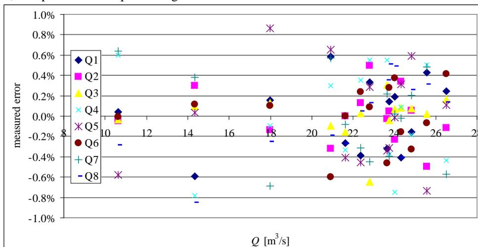
Figure 4: Errors in  $Q_i$  for single time series.
