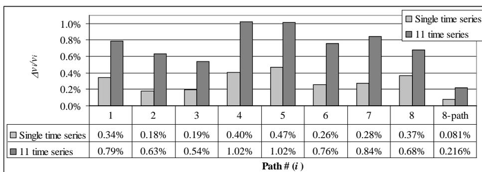
Figure 5: Random errors for velocities measured in 2008 showing the mean errors of the single time series and the spread of the 11 time series.
