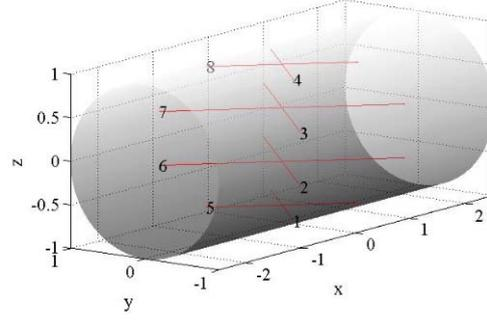
**Figure 2 : Enumeration of acoustic paths. The flow is along the positive direction of the  $x$ -axis, and the  $y$ -axis is horizontal.**
