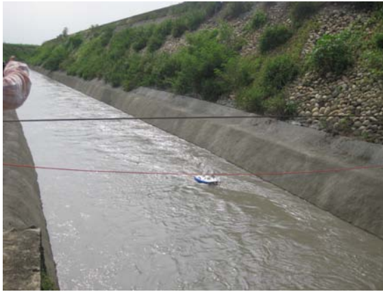
Fig. V: Q Measurement using Riversurveyor
