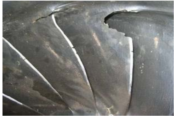
Fig. 8 Erosion of runner at the out let during the operation period of 1 year at JHC (Courtesy, BPC)
