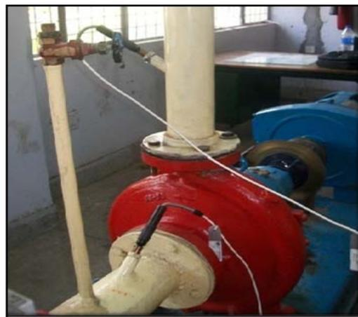
**Fig.2. Thermowells and thermometers at the inlet and outlet of the turbine**
