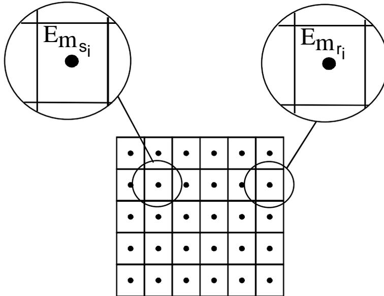
Figure 5. Cross-sectional grid in draft tube outlet.
