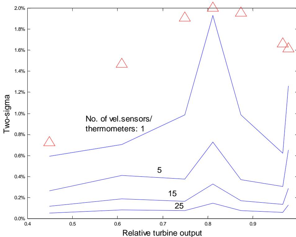
**Figure 8. Computed error levels for 1, 5, 15 and 25 probe positions in the 5 by 6 point grid of the cross section, as a function of the turbine output. The highest error level occurs at best-efficiency point of operation. Efficiency curve is out of scale.**
