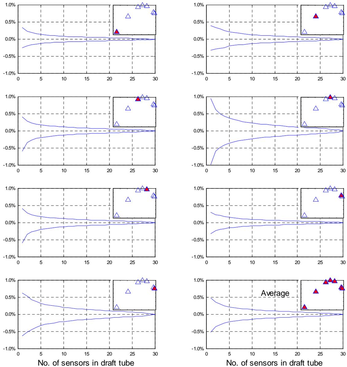
**Figure 7. Results from calculating the 95 % confidence levels for ‘n’ probe locations, ‘n’ covering the range from 1 to 30 locations in the 5 by 6 point grid of the cross section. Each plot is from a single operational point of the turbine, indicated by the relative P- $\eta$  curve.**
