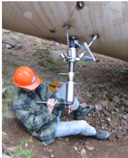
Figure 4: The screw-in process of the transducer
