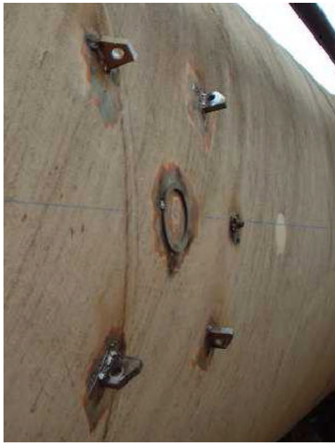
Figure 3: Weld on lugs and centering ring temporary welded as well as installed acoustic screw-in transducer.
