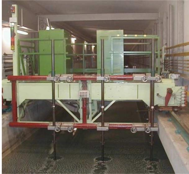
Figure 2: The towing vehicle with the 3 mounting rods.
