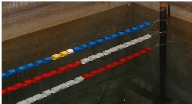
Figure 6: Wave-breakers mounted at both ends of the tow tank.
