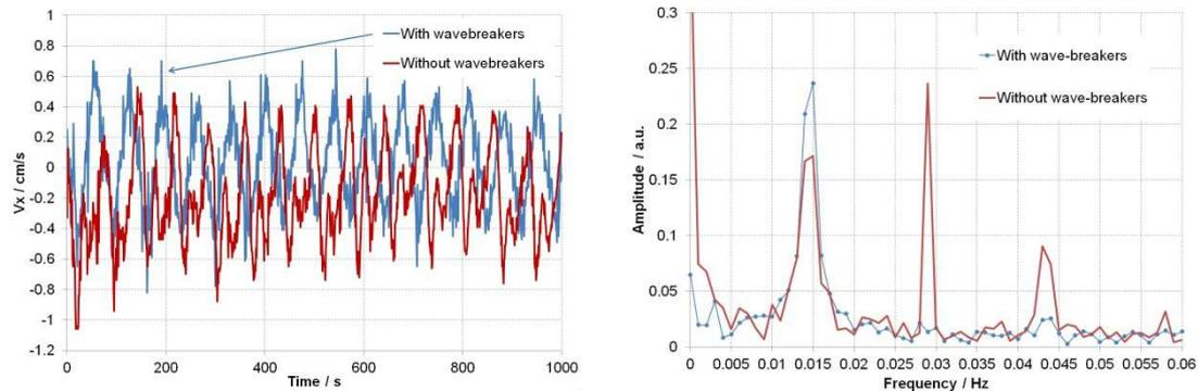
Figure 7: Left) Residual velocity after a run at 1 m/s with and without wave-breakers. Right) Associated Fourier spectra from the graph on the left.
