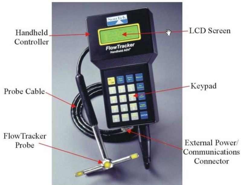
Figure 3: FlowTracker with 2D Side Looking Probe, taken from [4]
