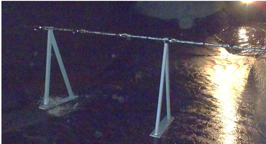
Figure 4 Arrangement of 7 current-meters in one fixed horizontal position for simplified measurements
