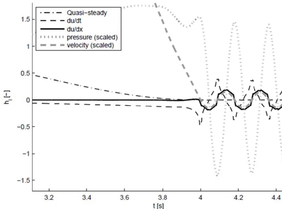
Figure 3: Simulated valve closure, with the differential pressure and velocity together with the friction due to each term in the Brunone model.
