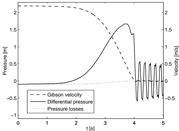
Figure 1: Example of a Gibson's integrated velocity with corresponding differential pressure and pressure losses. Data obtained from a simulated valve closure using a 1-dimensional model ( $Re=0.65 \cdot 10^6$ ,  $D=0.3$  m), Jonsson [3].
