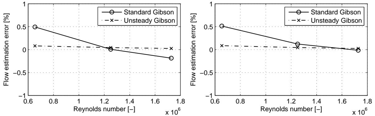
Figure 5: Deviation of the standard and unsteady Gibson-estimated flow rate relative the initial flow from simulations. Left figure corresponds to a test section length of 6 m and right figure to a length of 9 m.
