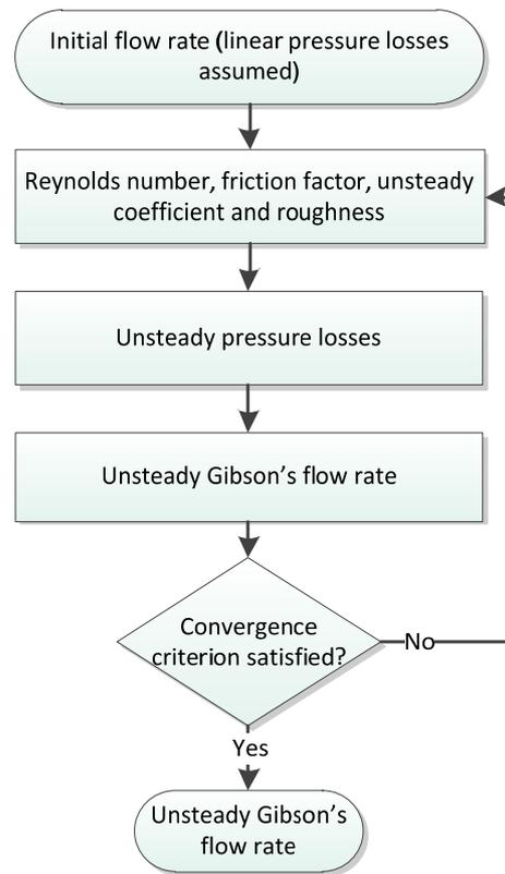
Figure 4: Procedure of unsteady Gibson's calculation.
