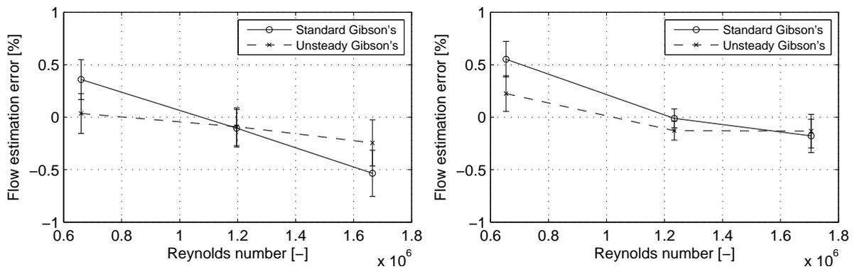
Figure 6: Deviation of the standard and unsteady Gibson-estimated flow rate from the reference. Left figure corresponds to a test section length of 6 m and right figure to a length of 9 m. The bars correspond to the uncertainty of the mean at the 95% confidence level.
