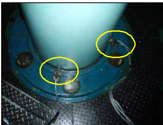
Fig. 7 – Vibration transducers setting on the turbine shaft
