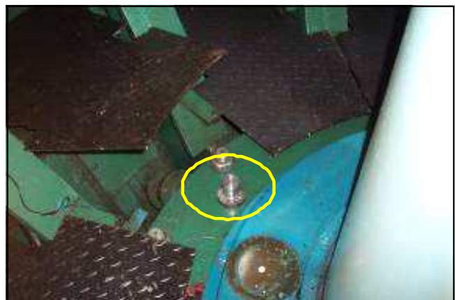
Fig. 8 – Accelerometer's location on the turbine cover
