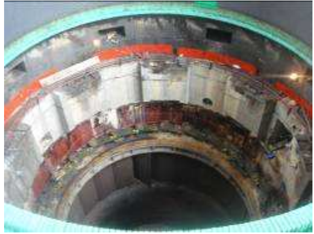
Fig. 4 – Generator stator and turbine guide vane
