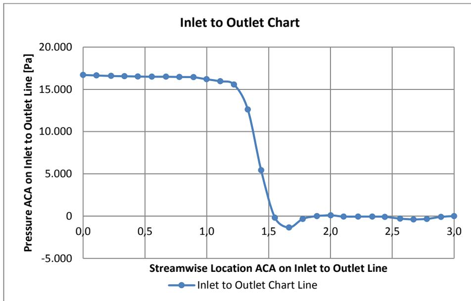
Figure 5 - Pressure on inlet, rotor and outlet domains.
