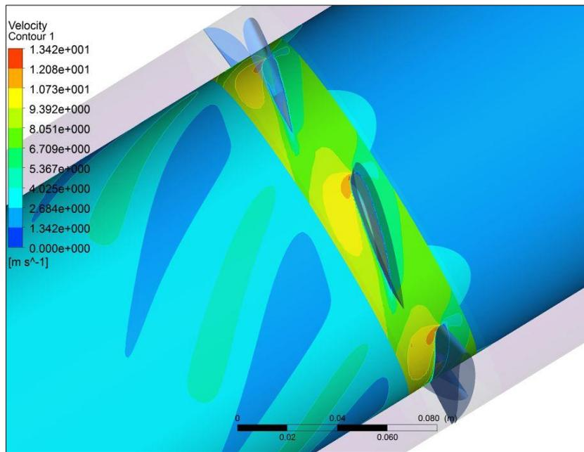
Figure 6 – Velocity contour at 50% span.
