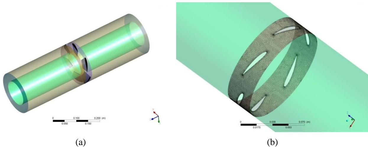
Figure 1 – (a) Assembled set mesh, (b) rotor domain mesh.
