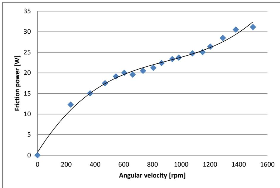
Figure 3 – Friction power.
