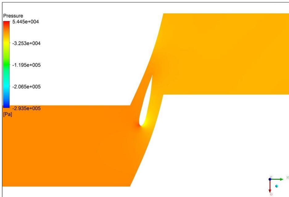
Figure 4 – Pressure on inlet, rotor and outlet domains, at 50% span.
