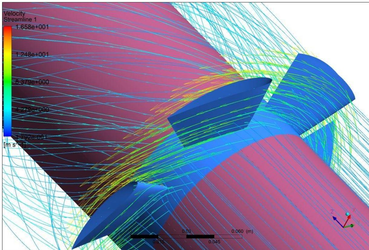
Figure 8 – Velocity vectors on the blades.
