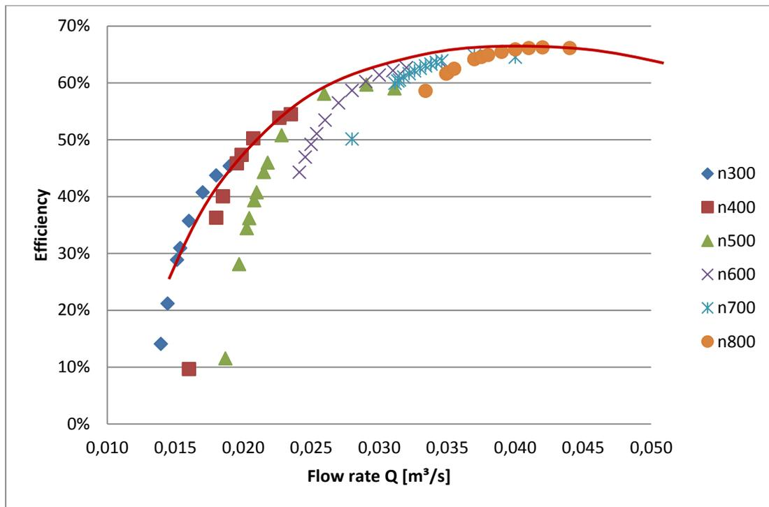
Figure 3 – Total Efficiency of the model of rotor.
