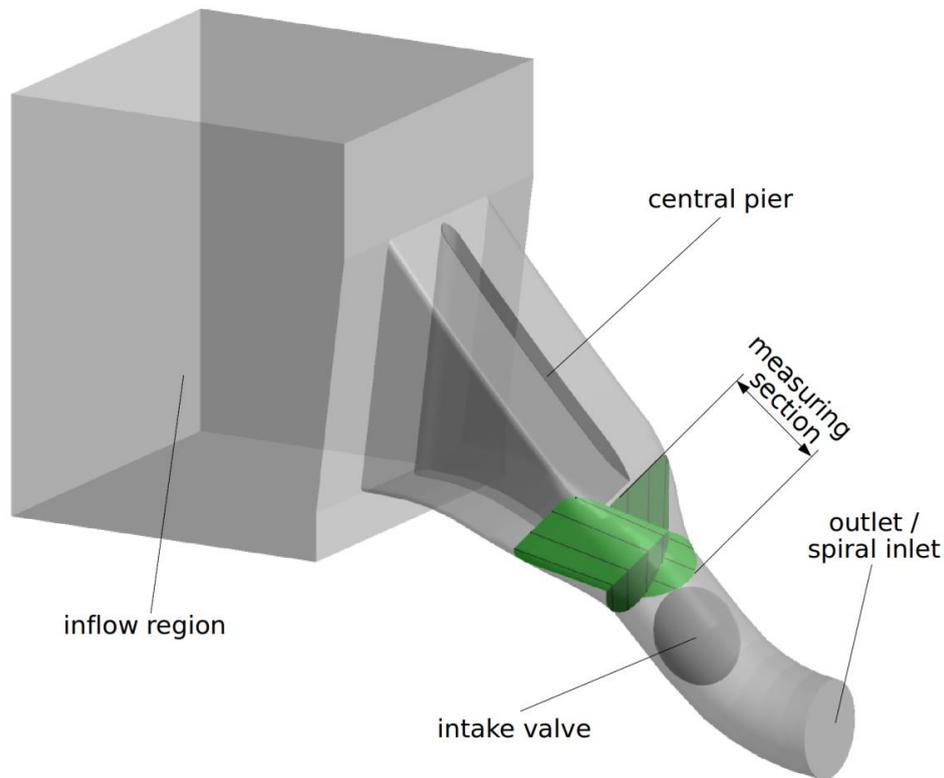
Figure 1 – Simulation domain of the turbine inlets and location of the measuring section
