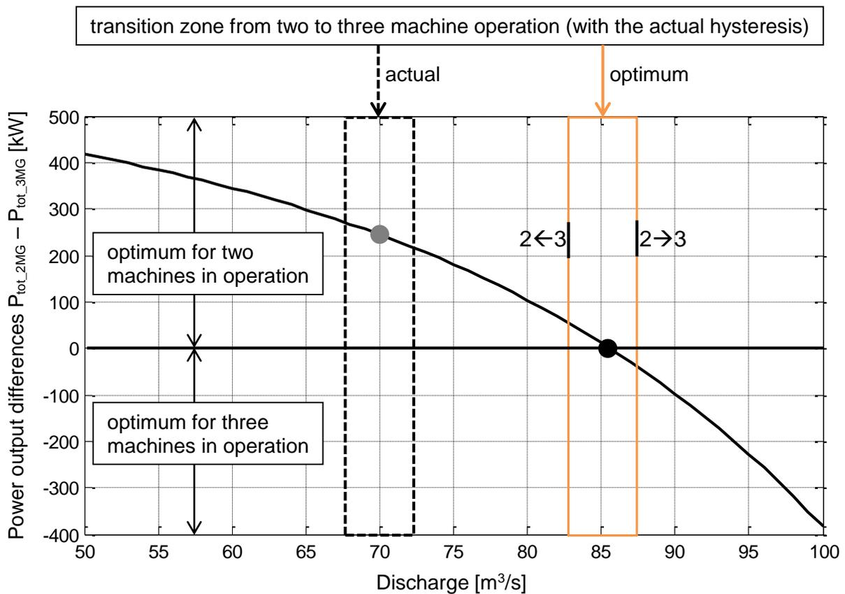
Figure 6 – Optimization of the discharge for the switching of the three machine operation
