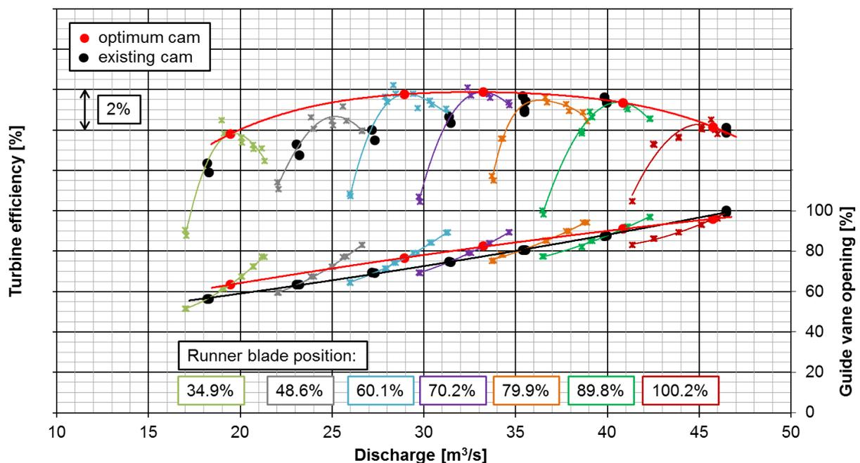
Figure 2 – Turbine efficiency for machine group 1 at the HPP Wettingen
