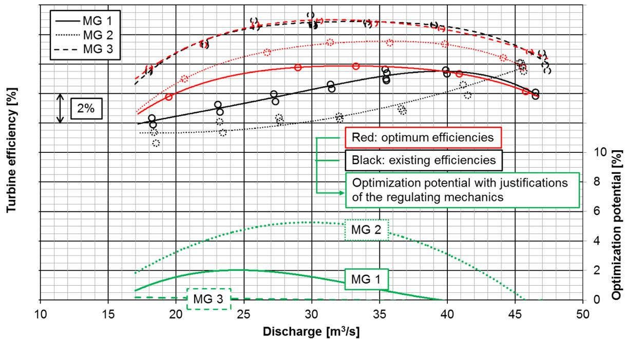
Figure 3 – Optimization potential for optimum cam operation
