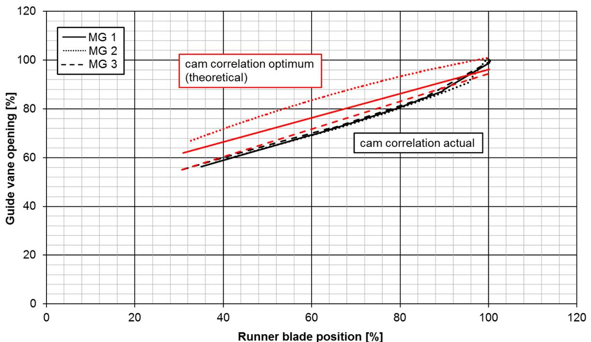
Figure 4 – Cam correlation analysis after the first measurement campaign
