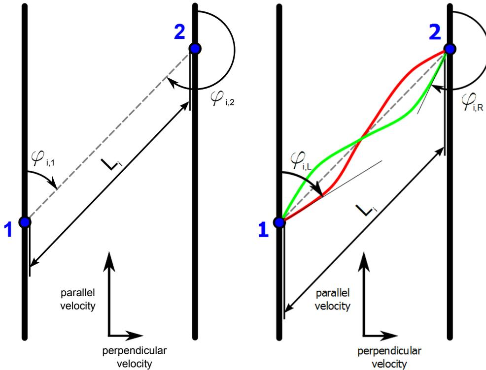
(a) Theoretically ideal acoustic path (gray dashed line), parallel velocity  $v_{\parallel}$ , perpendicular velocity  $v_{\perp}$ , acoustic path length  $L_i$ , left path angle  $\varphi_{i1}$  with respect to the conduit axis, right path angle  $\varphi_{i,2} = \varphi_{i1} + \pi$  (source: [8]).
