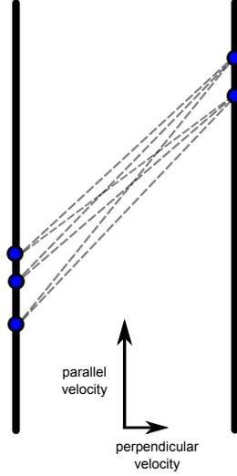
Figure 3: Geometry of multiple acoustic paths in close-by arrangement: This example shows  $n_1 = 3$  sensors on the left and  $n_2 = 2$  sensors on the right spanning an acoustic plane with  $n = 6$  paths (source: [8]).
