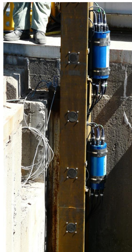
Figure 3: Frame supporting the ASFM transducers
