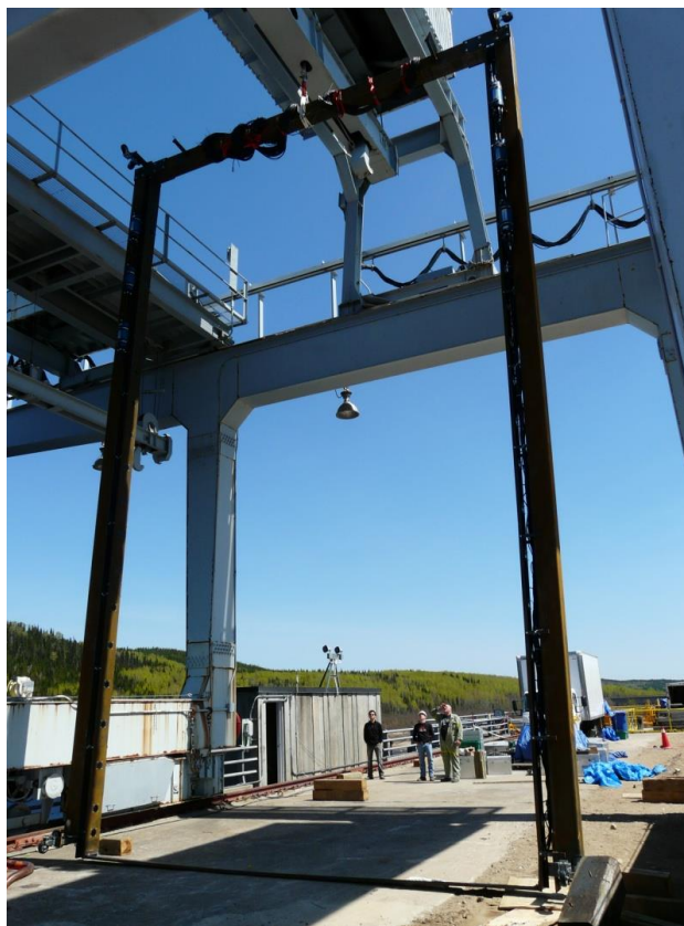
Figure 3: Frame supporting the ASFM transducers
