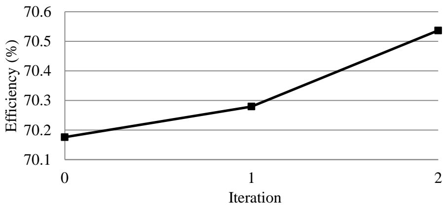
Figure 12 – Efficiency evolution during the optimization process – 18 MW.
