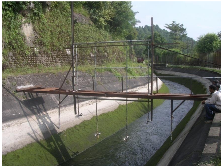
Figure 5 – Current Meter Mounting Structure used at Power Channel for Discharge Measurement
