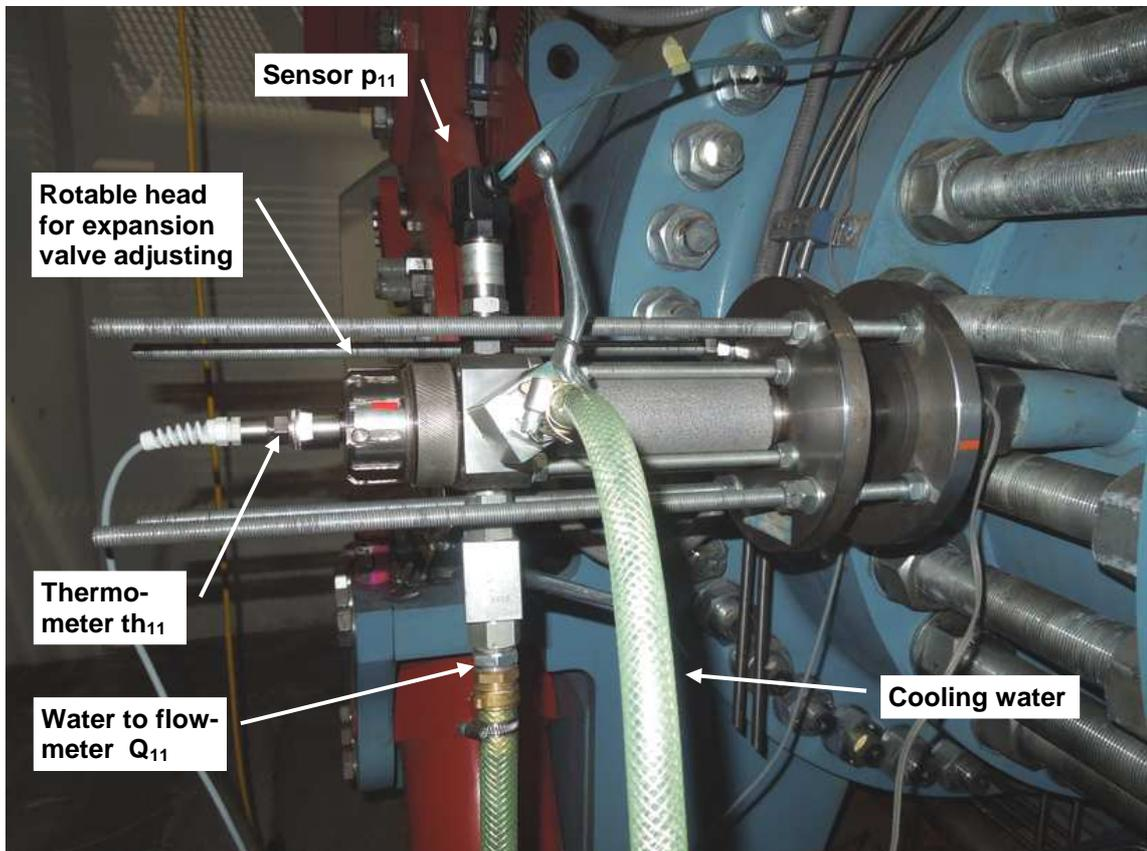
Fig. 3 Thermodynamic sampling probe in the high pressure profile
