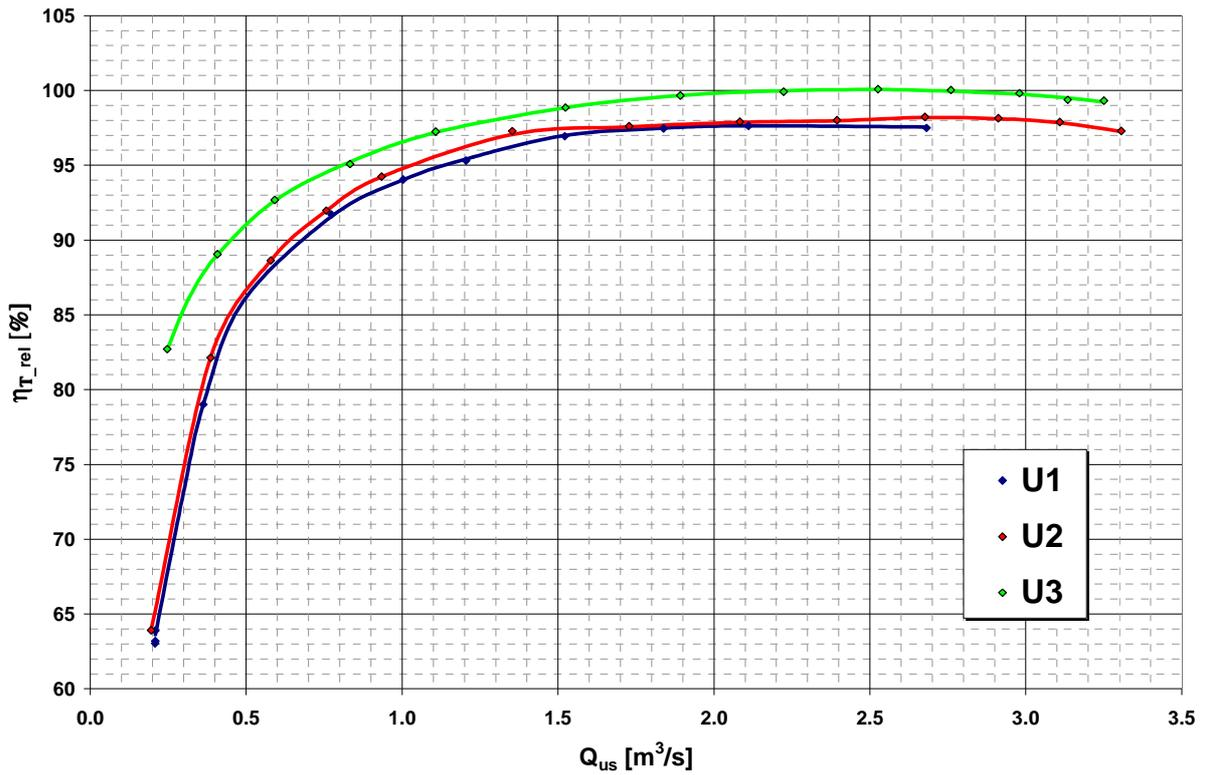
*Fig. 5 Turbine efficiency determined by thermodynamic method*
