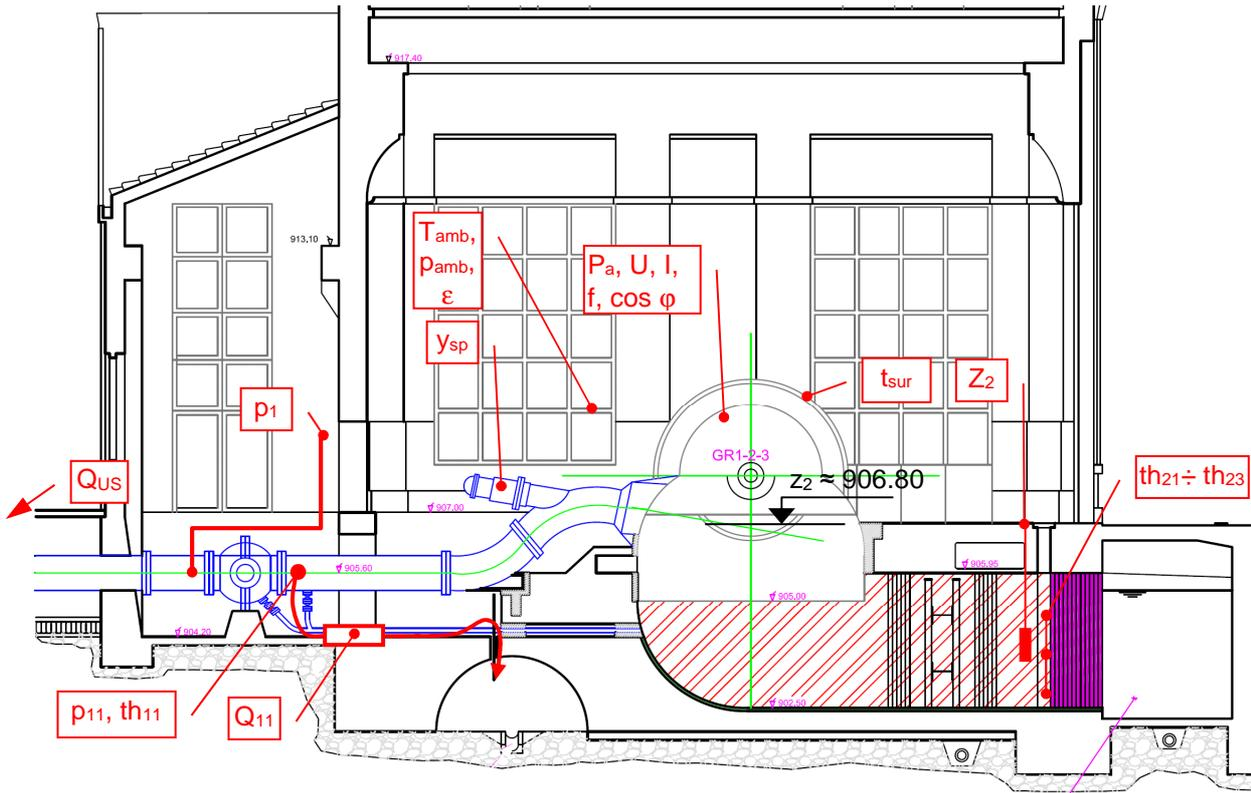
Fig. 2 Location of the main sensors used for the unit performance tests
