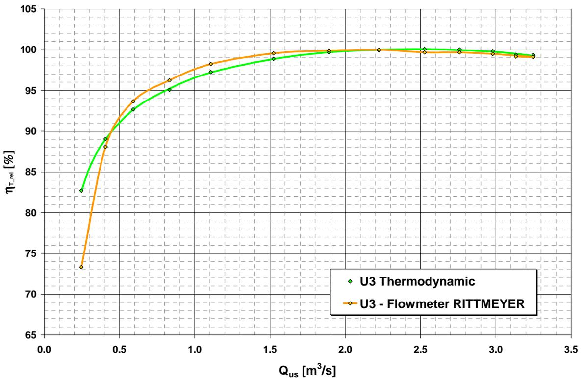
*Fig. 6 Efficiency curves as determined by thermodynamic and by indirect method*
