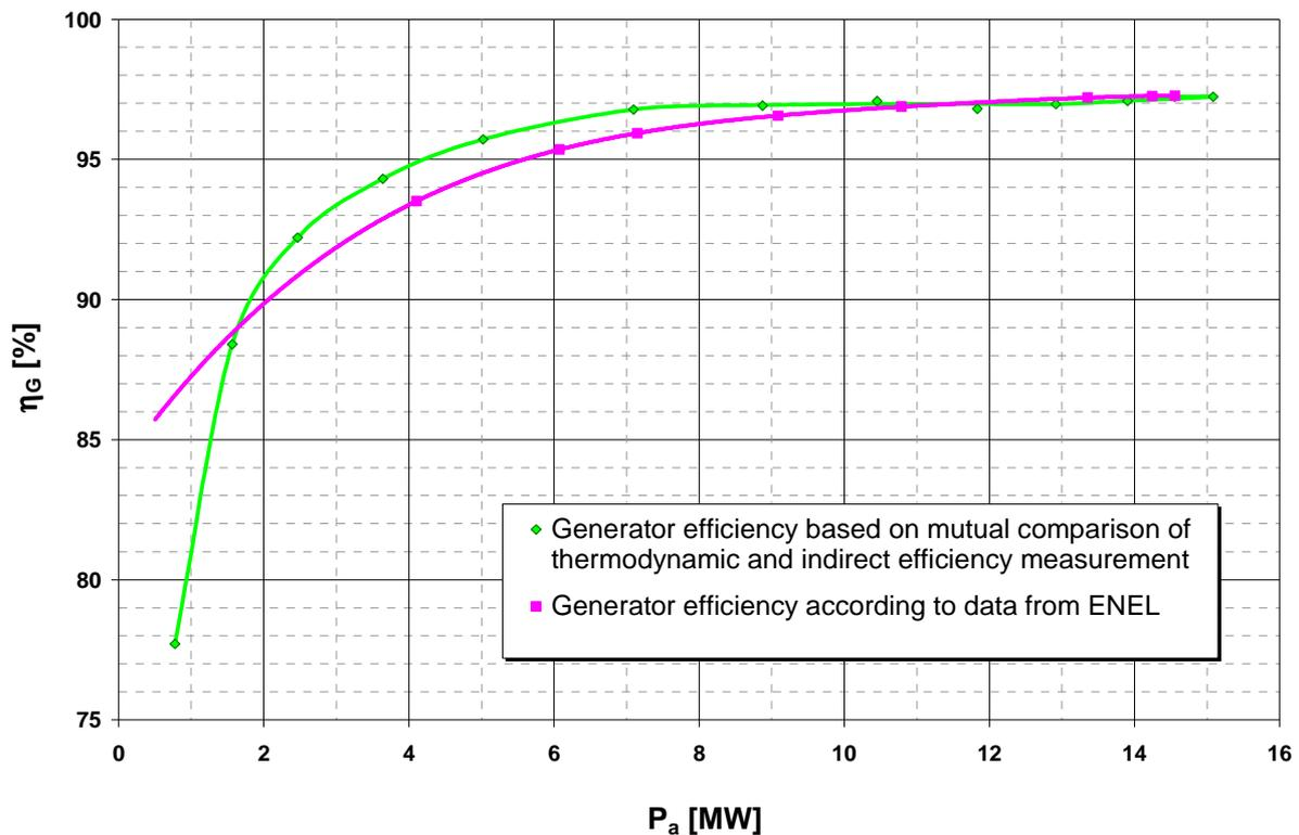
*Fig. 7 Comparison of generator efficiency curves*
