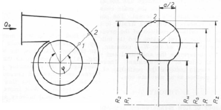
Figure 3: location of pressure taps 1 and 2 shown for WK method [4]
