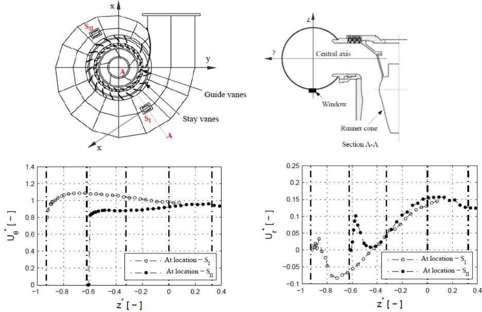
Figure 8: Tangential and radial velocity from LDA measurement from [37] in the spiral case of Kaplan turbine.
