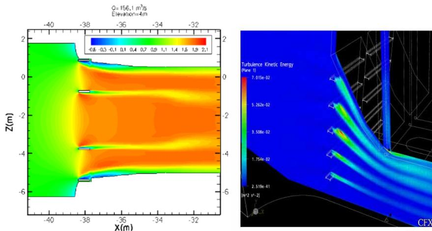
Figure 6: velocity component distribution due to trash racks [26] and turbulent kinetic energy distribution after trash rack [27]
