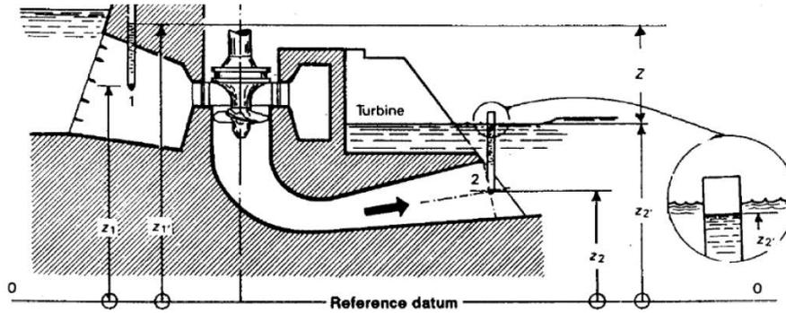
Figure 1: Measurement points for Low head turbine (Kaplan turbine) [4]
