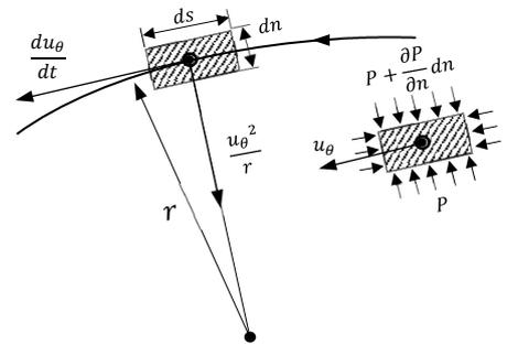
Figure 2: Streamline coordinates and forces acting
