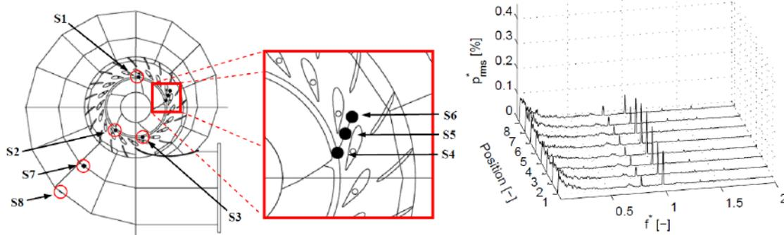
Figure 9: Amplitude spectrum at spiral case (*right*) for the sensors mounted in casing (*left*) [50]
