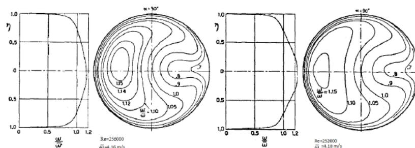
Figure 7: Effect of inlet velocity profile (secondary flow) in velocity distribution in sectional plane of curved pipe. [30]
