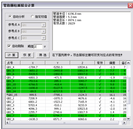
(a) Fitting Process of Cylindrical Surface
