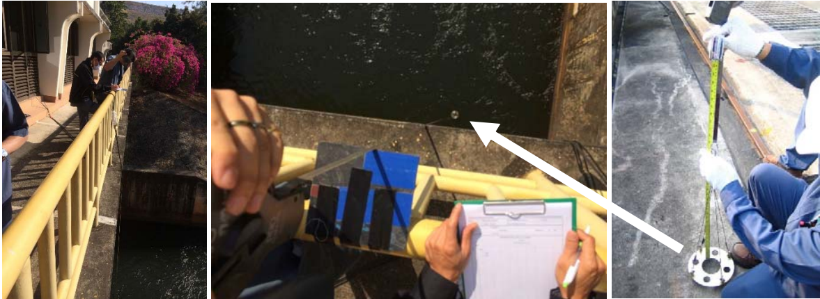
Figure 9: Measuring Tailrace Water Level by Measuring Tape with Plate Gauge
