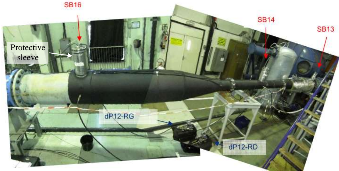
Figure 5: Photograph of the test section and its insulation
