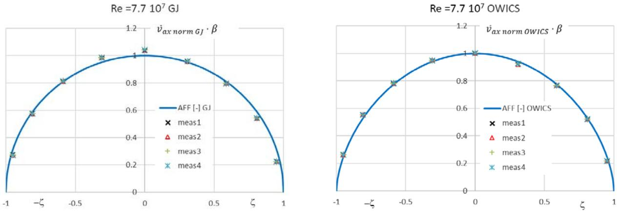
**Fig. 6:** Case 3, normalized measured AFF data, a) vs. Gauss-Jacobi AFF, b) vs. OWICS AFF
