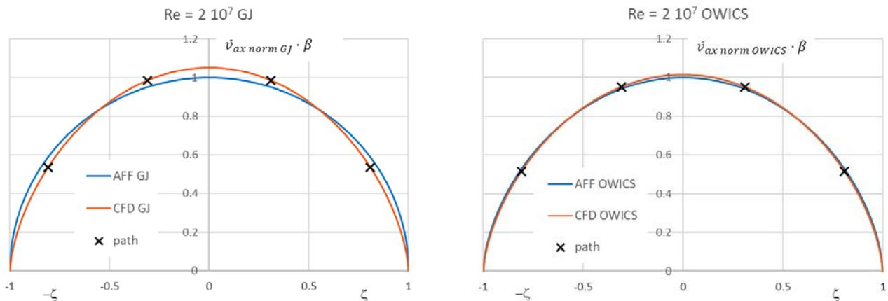
**Fig. 4:** Fully developed a) normalized CFD AFF vs. Gauss-Jacobi AFF, b) normalized CFD AFF vs. OWICS AFF
