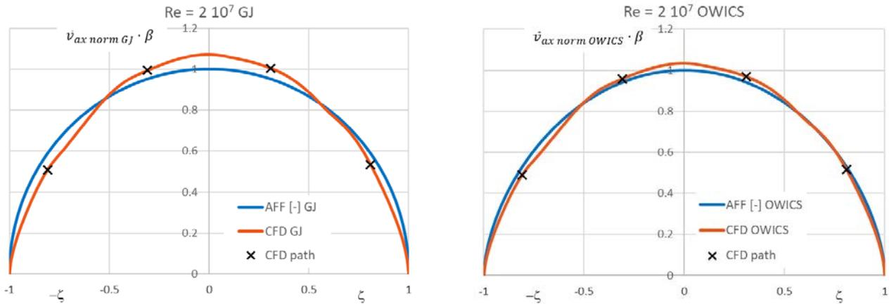
**Fig. 7:** Case 4, a) normalized CFD AFF vs. Gauss-Jacobi AFF, b) normalized CFD AFF vs. OWICS AFF
