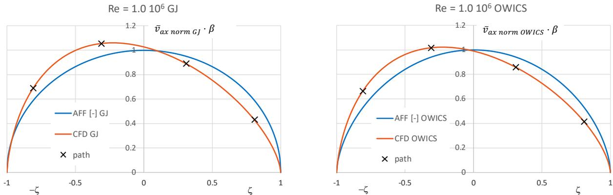
**Fig. 4:** Case I, a) normalized CFD AFF vs. Gauss-Jacobi AFF, b) normalized CFD AFF vs. OWICS AFF
