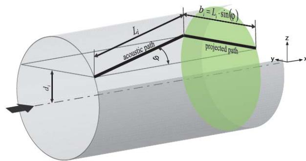
**Fig. 2:** Projection of the acoustic path of the partial flow rates on the y-z-plane ( $d_i = \text{abs}(z_i)$ )
