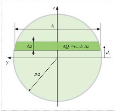
**Fig. 1:** Integration by summing up ( $d_i = \text{abs}(z_i)$ )
