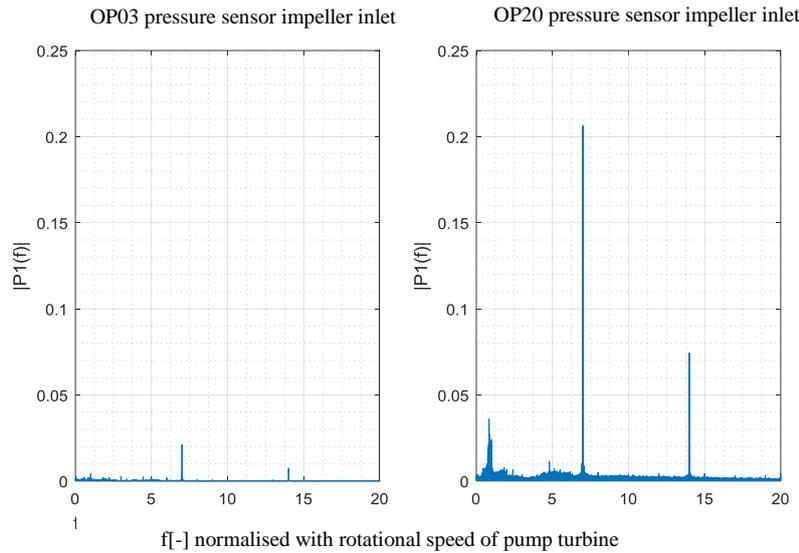
**Fig 3:** Frequency spectrum of transient pressure sensor (impeller inlet) without (left) and with (right) swirl
