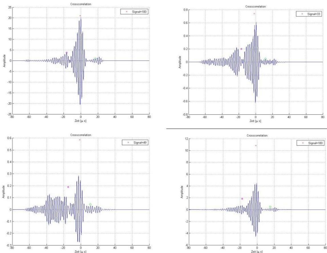
**Fig 7:** samples of correlation functions: upper left undisturbed signal, other signals: different degree of disturbance
