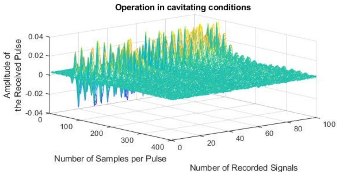
**Fig. 5:** Ensemble of signal shape (amplitude) of the recorded ultrasonic pulses over time under cavitating conditions
