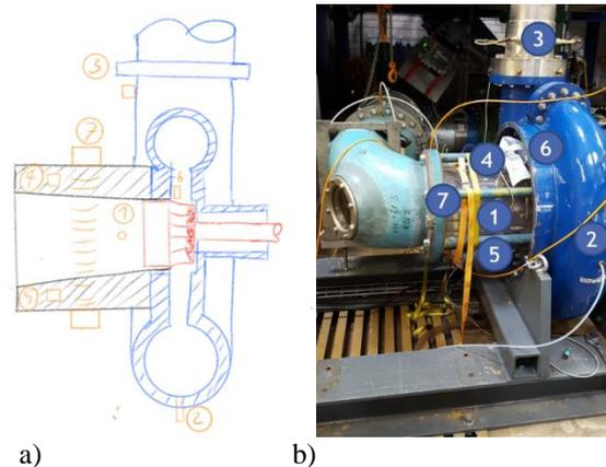
**Fig.1.** a) schematic drawing of turbine with transient measurement positions b) photo of the pump turbine test rig
