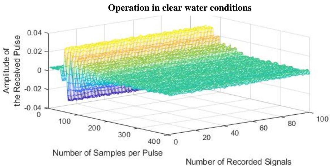
**Fig. 4:** Ensemble of signal shape (amplitude) of the recorded ultrasonic pulses over time for clean water conditions
