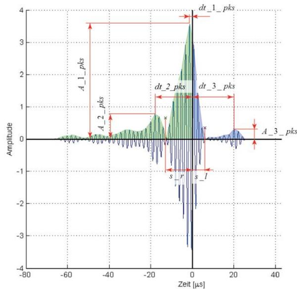
**Fig. A2:** correlation function with characteristic parameters
