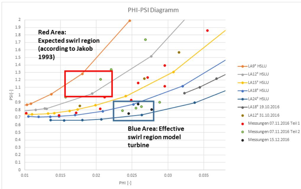
**Fig. 2:** Characteristic curves for constant guide vane (LA) opening in the  $\Phi$ - $\Psi$ -plane and the operating points for the measurement campaigns, measurement points indicated by single colored dots, red area swirl region from [7]
