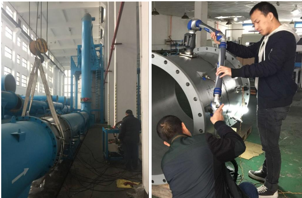
(a) large-diameter flowrate standard facility (b) geometrical measurement using FARO arm Fig. 3: photos of laboratory test
