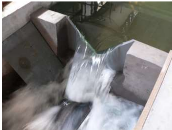
Figure 3: Typical flow patterns (weir head is 40.08cm).
