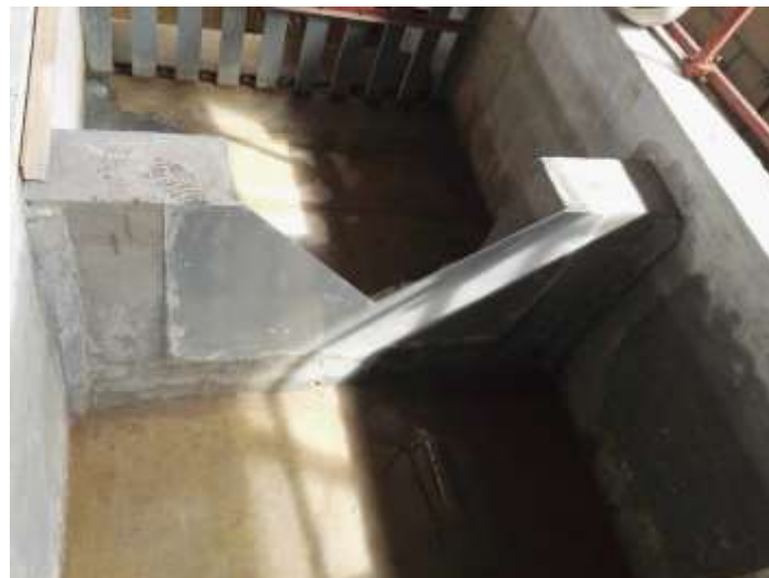
Figure 2: Triangular sharp-crest weir.
