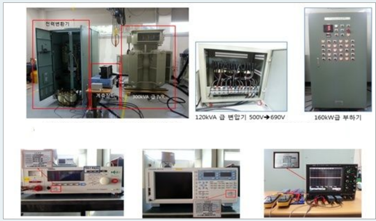
Performance testing equipment for a power converter
