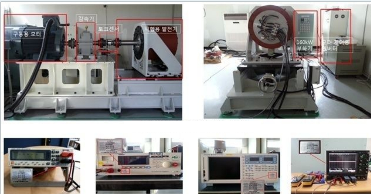
150kW dynamo testing system
