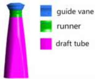
Figure. 1 Draft tube model
