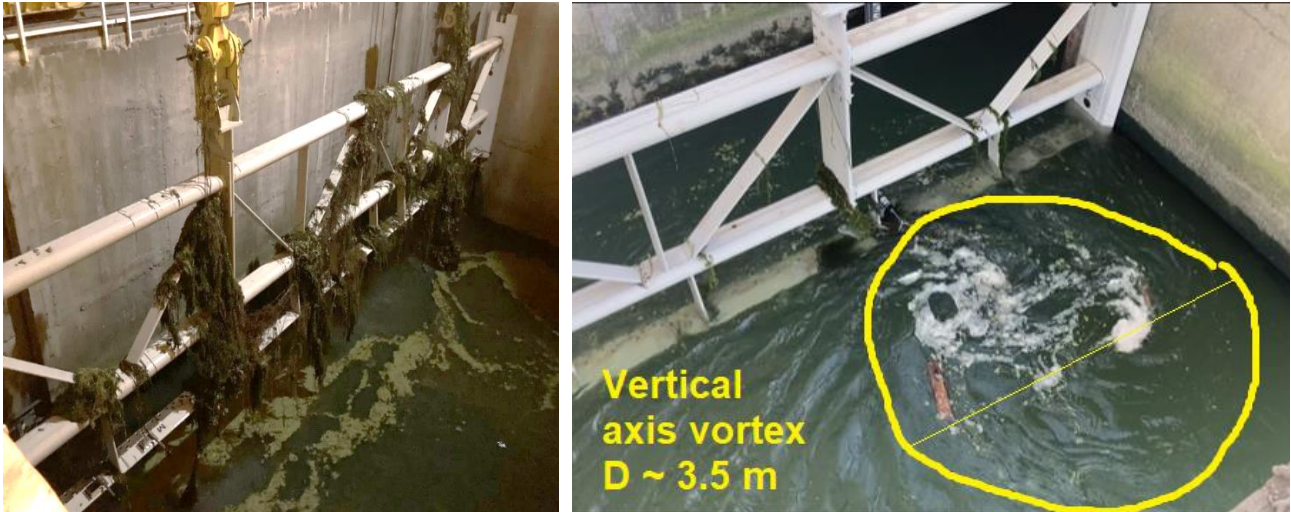
Figure 1: Left) River vegetation entangled on the measurement frame; Right) Vortex structure on the right side of the A7 turbine inlet
