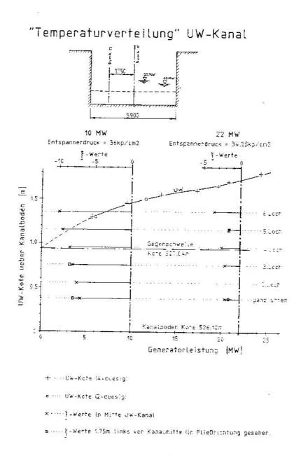
The open channel was measured in 2 sections and 6 levels.
