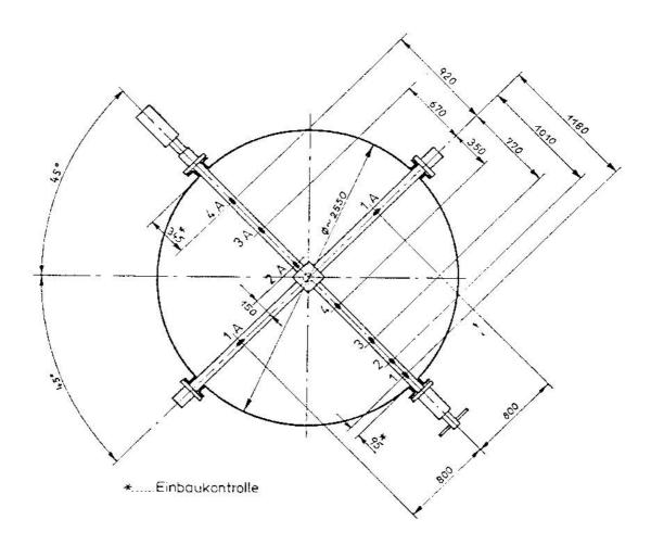
With the above shown arrangement each opening can be used separately to take off water from the draft tube. Only the two openings "1A" are connected and the water out of these two openings is mixed. The check of the different measuring point was done at 72 and 180 MW output. The differences in the reading of the bridge are a measure for the temperature difference.
