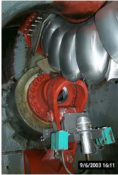
Figure 10: Camera and strobelsights for jet visualisation
