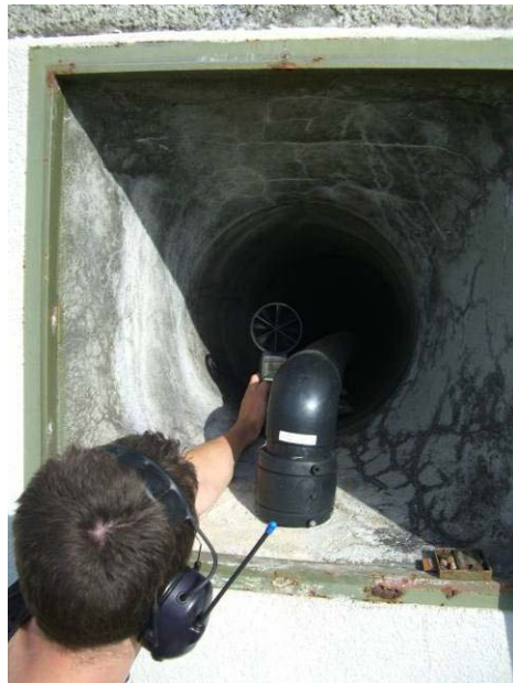
Fig.10: Temperature and air velocity measurements at the inlet of the air aspirated by the Pelton Turbine
