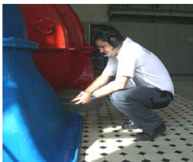
Fig. 8: Relative humidity measurement close to the heat exchanging wall
