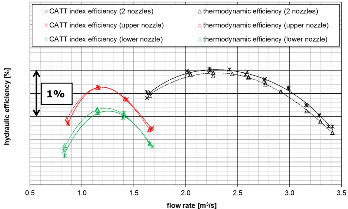
Fig. 20: Comparison between thermodynamic efficiency and CATT index efficiency
