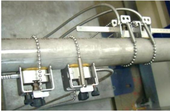
Fig. 6: CATT measurement at  $D_i=50$  mm pipe
