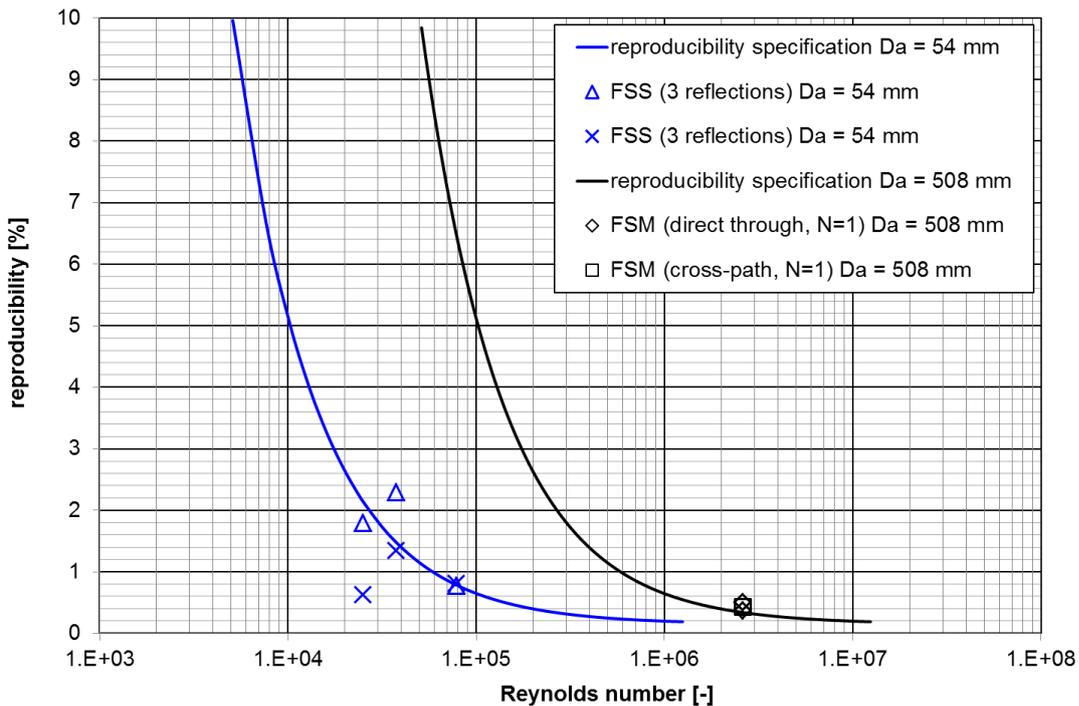
Fig. 10: Reproducibility of CATT measurements under varying Reynolds number
