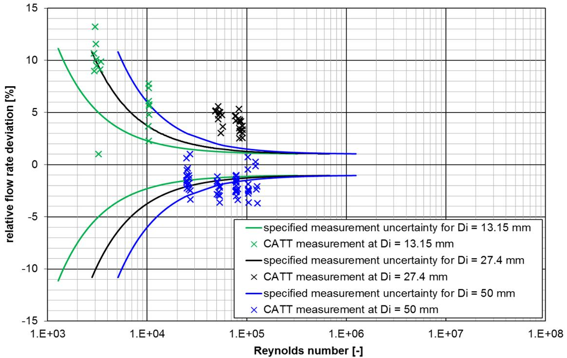
Fig. 12: Relative deviations with the FSS transducer
