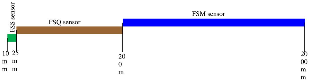
Fig. 15: Appropriate internal pipe diameter range for the FSS, FSQ and FSM transducer
