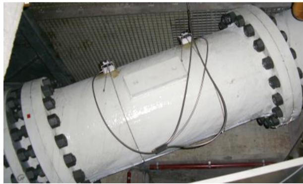
Fig. 7: CATT measurement at HPP Sassello
