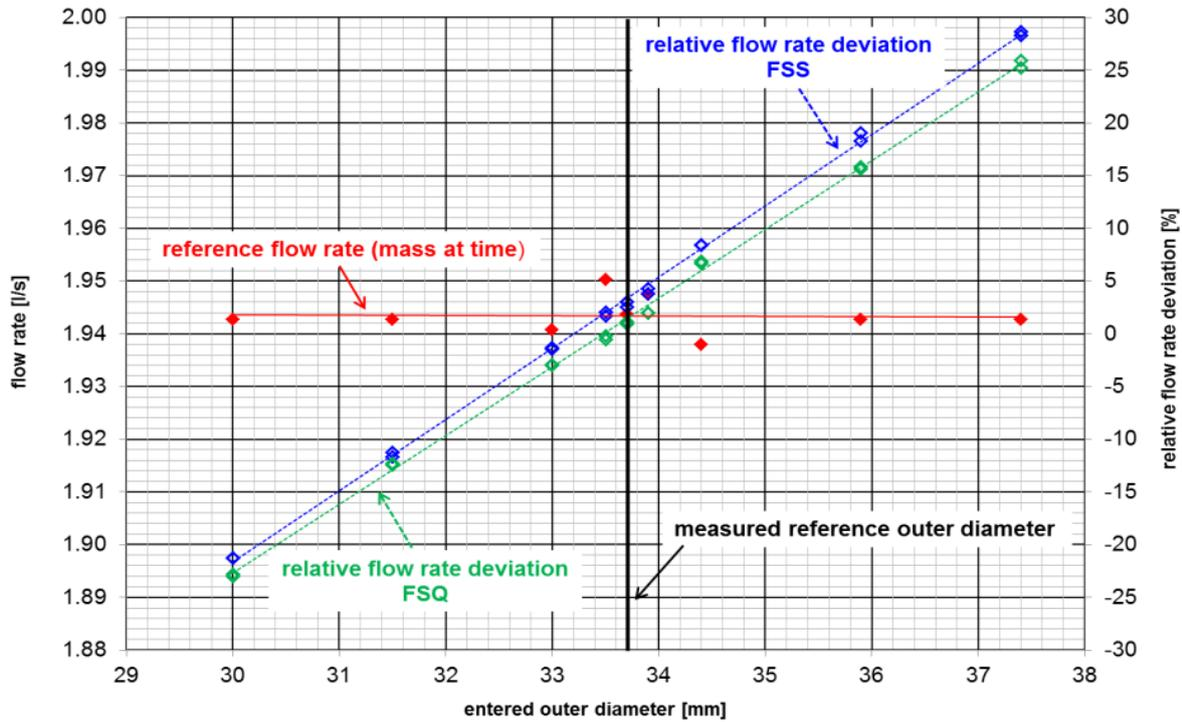
Fig. 16: Relative deviations in function of varying diameter
