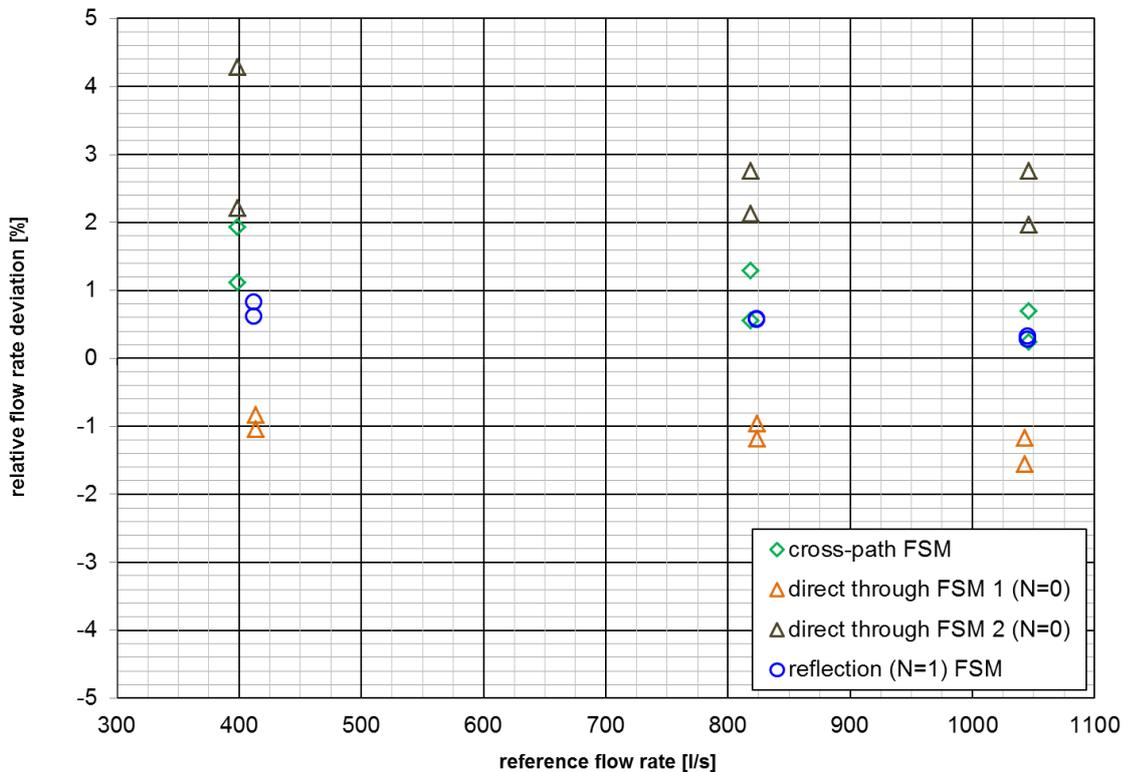
Fig. 8: CATT measurements at  $D_i=502.9$  mm pipe with various installation arrangements
