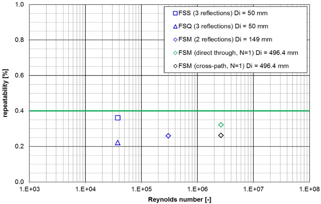
Fig. 9: Repeatability of CATT measurements under varying Reynolds number
