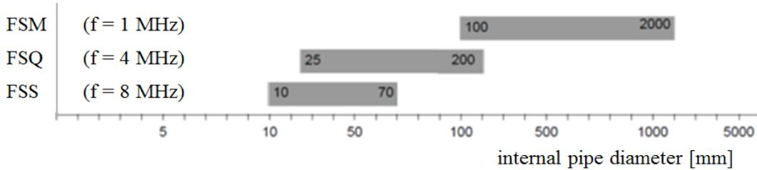
Fig. 1: Specified application range of the three transducer pairs
