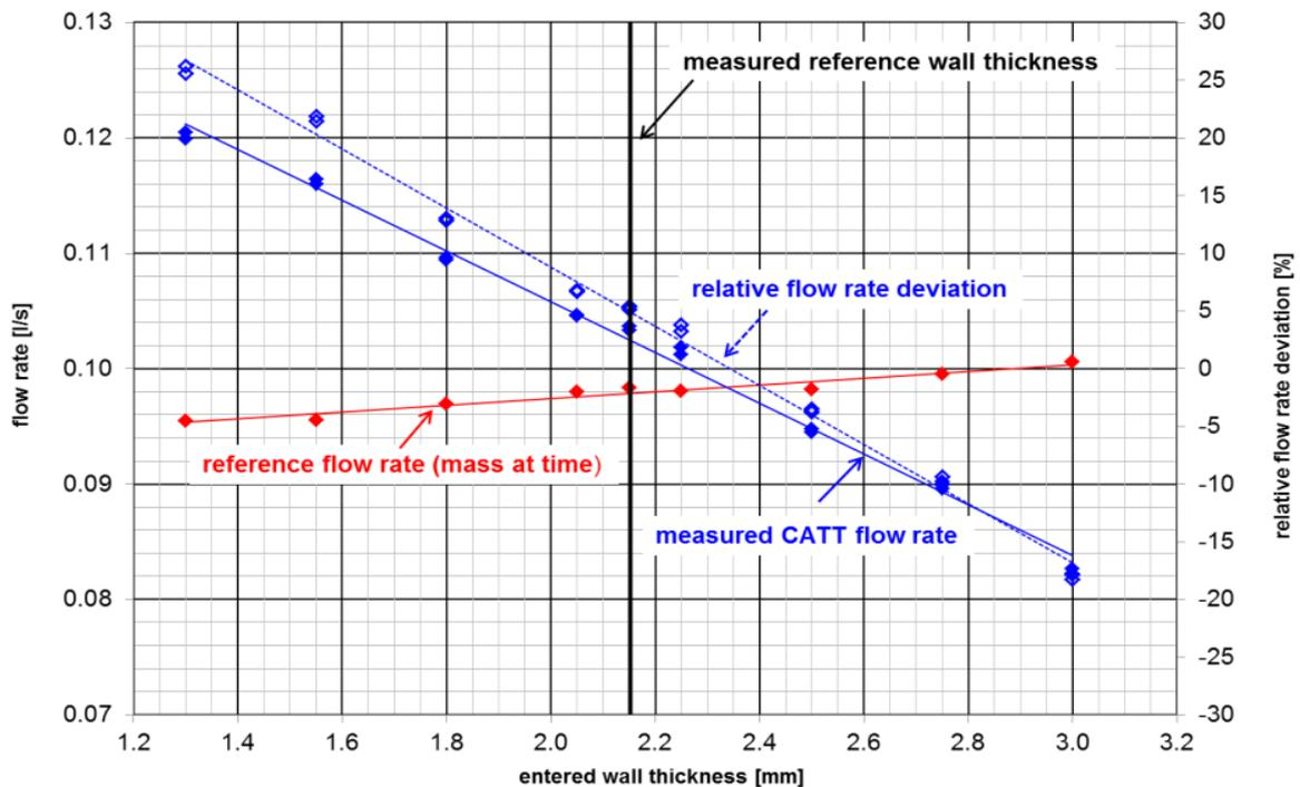
Fig. 17: Relative deviations in function of varying wall thickness
