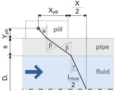
Fig. 5: Scheme for the pill to pill separation calculation
