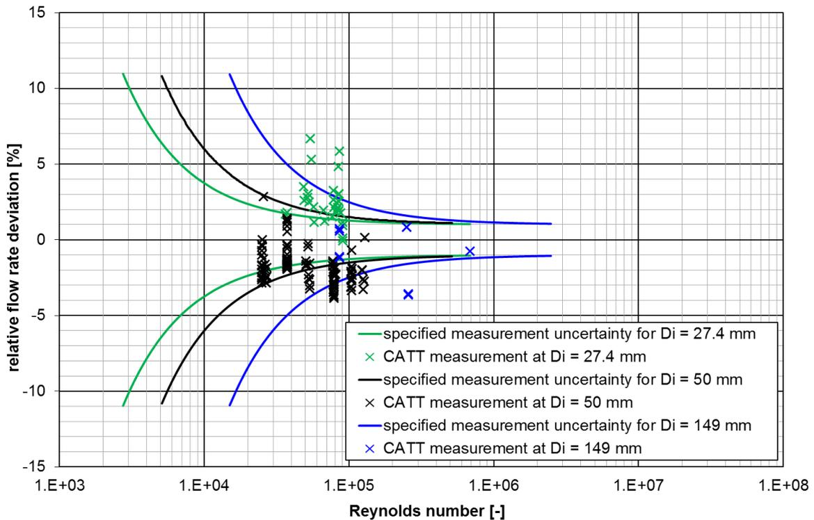
Fig. 13: Relative deviations with the FSQ transducer
