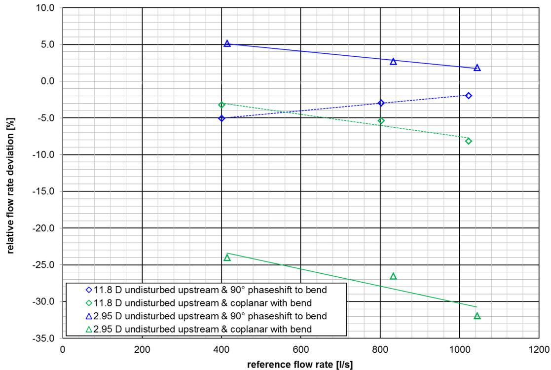
Fig. 18: Influence on relative flow rate deviation by upstream disturbances
