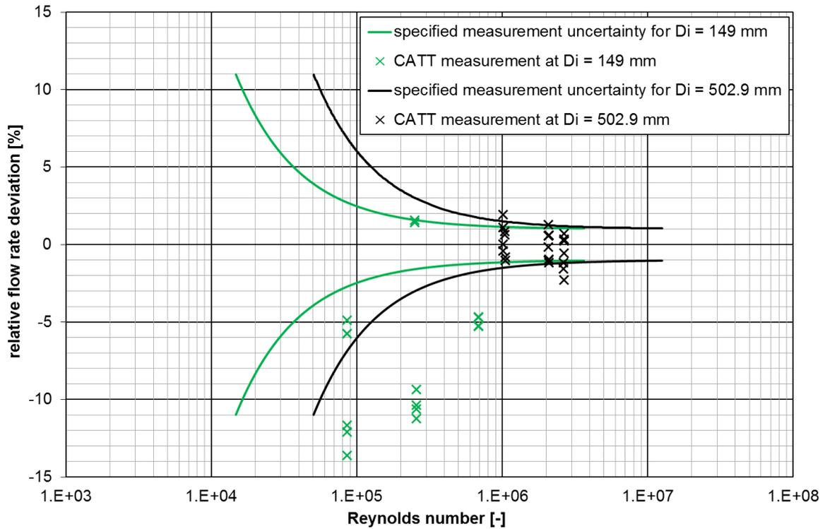
Fig. 14: Relative deviations with the FSM transducer
