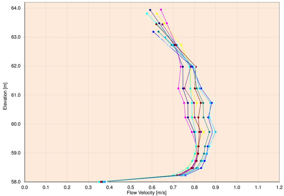
(b) Main axial velocity profiles of different headwater levels: The total discharge remains quite constantly over the whole operating range. Only the profile is getting bulgier with lower head.
