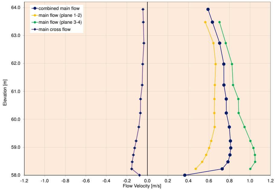
(a) Flow profile at maximum headwater level: cross flow  $\bar{v}_\perp$  (blue diamonds), main axial flow  $\bar{v}$  (blue circles), axial flow obtained by plane 1-2  $v_1$  (yellow), and axial flow obtained by plane 3-4  $v_2$  (green)
