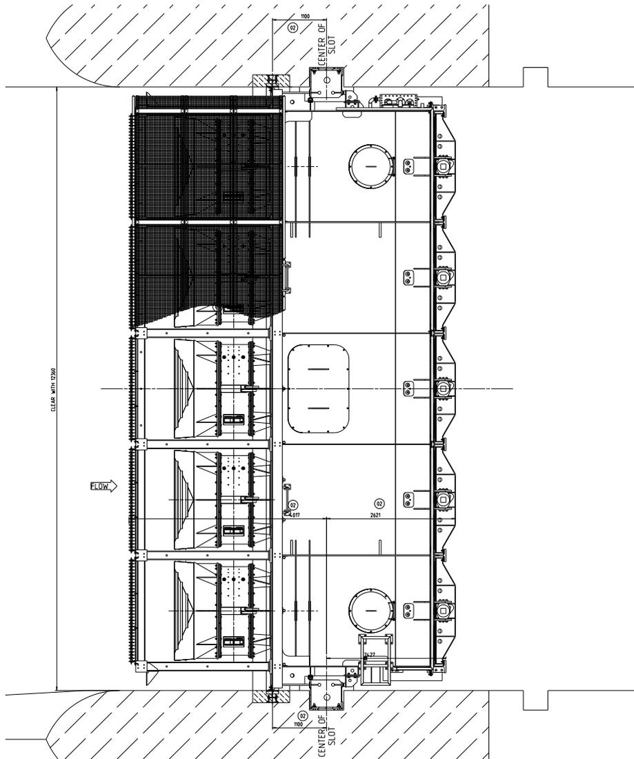
Figure 2: General layout of the HYDROMATRIX® module (plan view)
