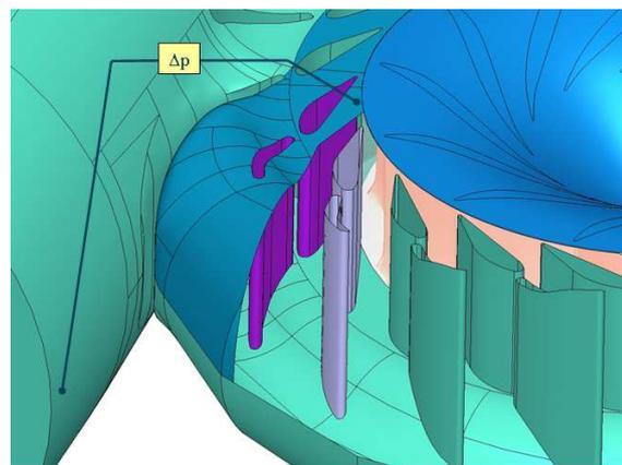
Figure 2 : Angular index installation on a Francis turbine
