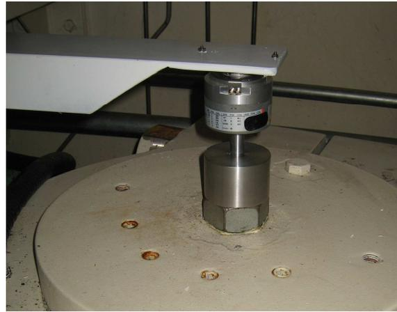
Figure 10 : Angular encoder attached to the guide vane axis
