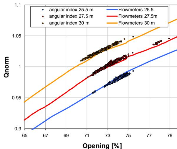
Figure 6 : Comparison of the flowmeter and angular index at various head
