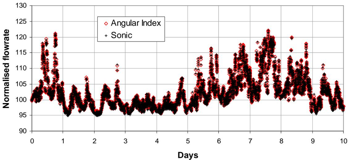
Figure 4 : 10 days of flowrate monitoring for the sonic and angular index method
