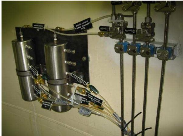
Figure 9 : Manifold for pressure mixing
