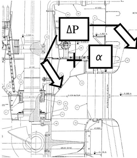
Figure 1 : Overview of the angular index measurement system on a propeller turbine
