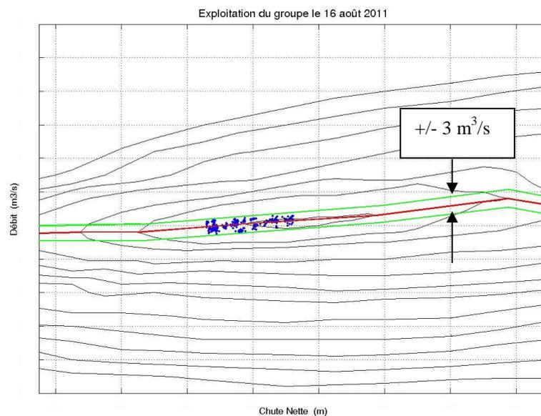
Figure 7 : Flow monitoring during optimal operation (head vs flowrate)
