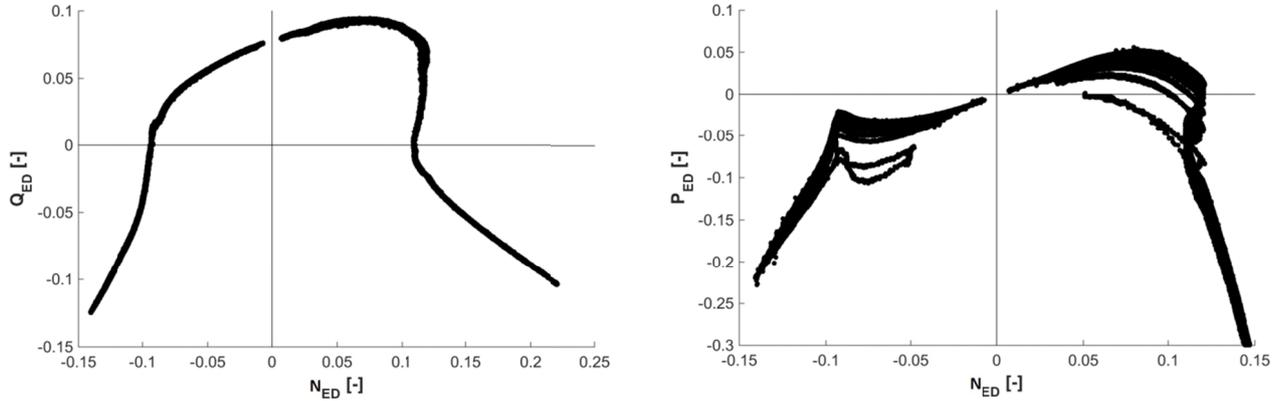
Figure 8. Resulting 4-quadrant characteristic curves of the PAT obtained with the dynamic measurements method.
