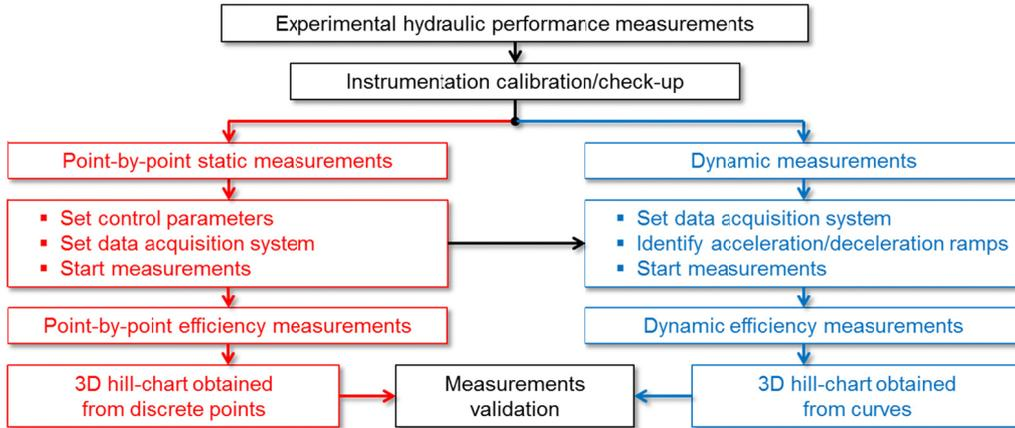
Figure 3. Flowchart of the employed experimental protocol, Hasmatuchi et al. [4].
