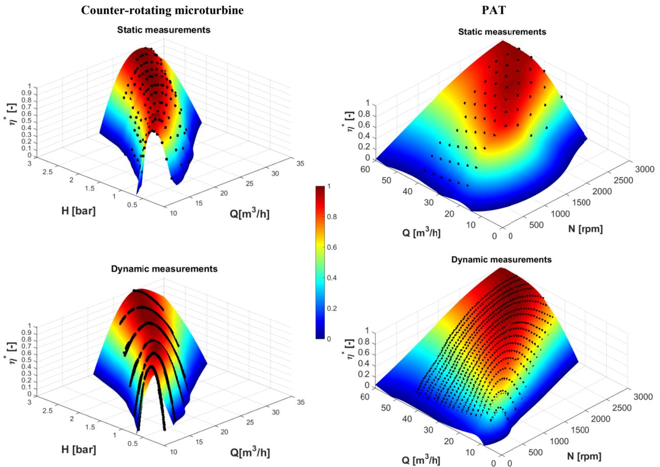
Figure 9. Resulting efficiency 3D hill-charts obtained by the classical static point-by-point and by the dynamic measurement methods.
