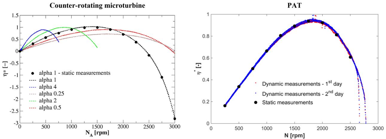
**Figure 7.** Comparison between dynamic and static efficiency measurements for fixed inflow conditions (recirculating pumps speed  $N_p = 1500/2000$  rpm).
