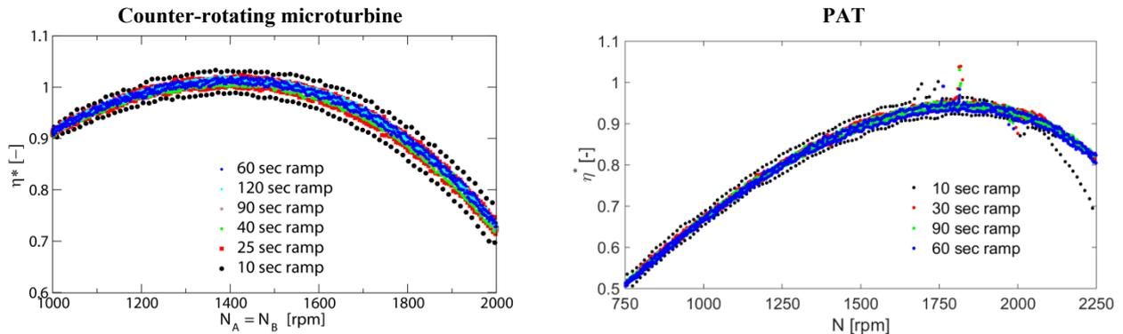
**Figure 4.** Influence of the acceleration/deceleration ramp of the runner(s) speed on the efficiency for fixed inflow conditions (pumps speed  $N_p = 1500/2000$  rpm).
