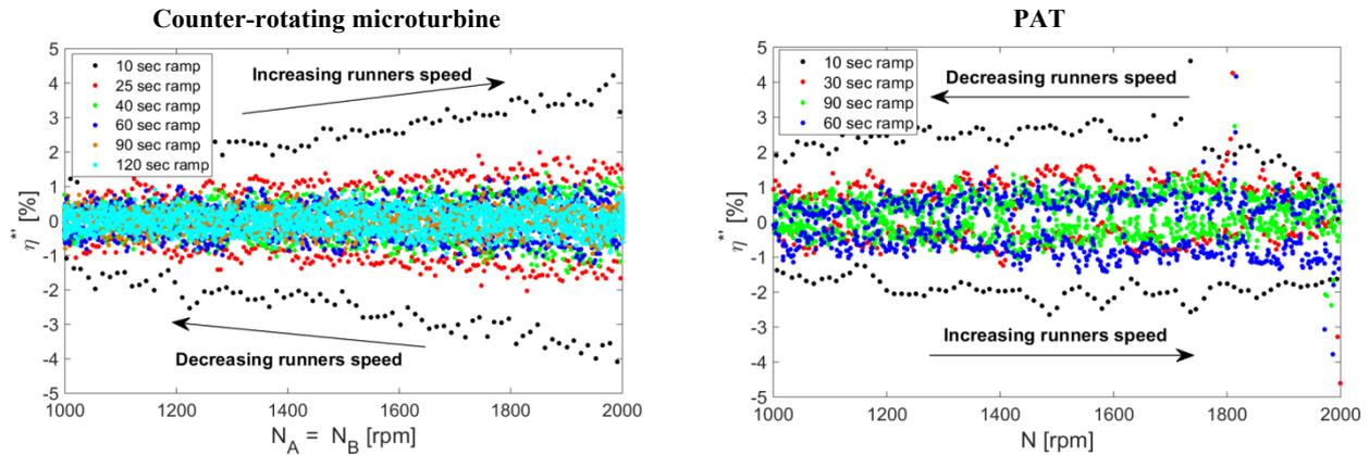
**Figure 5.** Efficiency fluctuation during an increasing/decreasing cycle at fixed inflow conditions (pumps speed  $N_p = 1500/2000$  rpm) for different speed acceleration/deceleration ramps.
