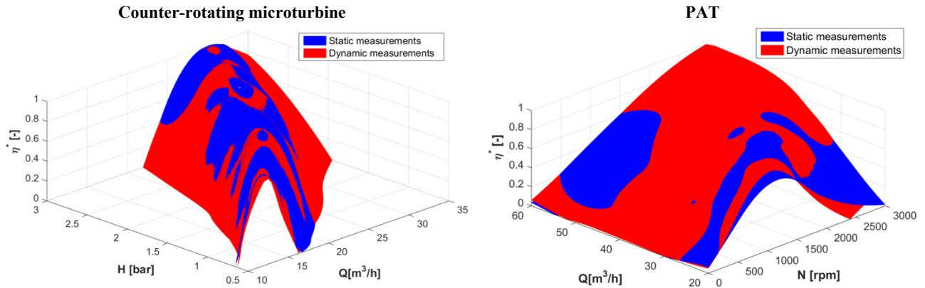
**Figure 10.** Validation of resulting 3D hill-charts obtained by the dynamic measurements method with the results of the classical static point-by-point method.
