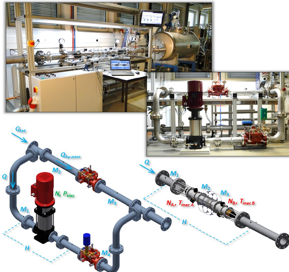
Figure 2. Experimental setup of the counter-rotating microturbine and of the PAT installed on the hydraulic test rig.
