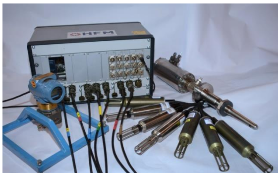
Figure 3: cRIO Measurement and Data Acquisition System
