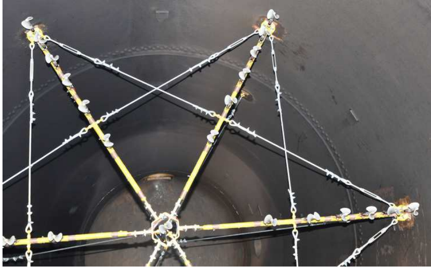
Figure 4 : Front view on the frame with current meters and MIV behind it
