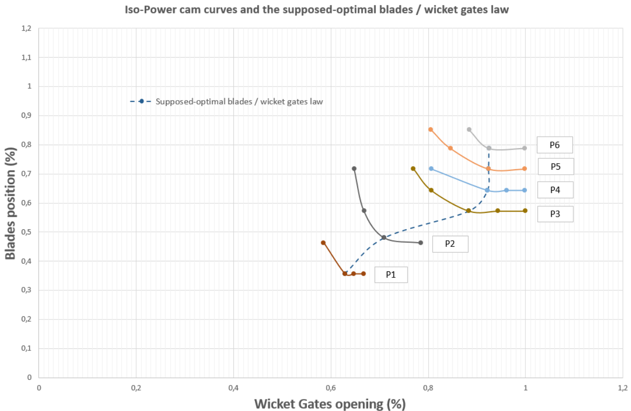
Figure 3: Graph from ancient but complete on-site test on one EDF’s unit for a given head
